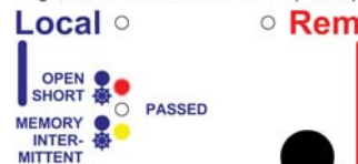
Fig 9. OPEN circuit at Pin 2 (Local)
