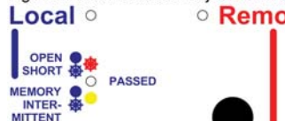
Fig11. SHORT between adjacent Pins
